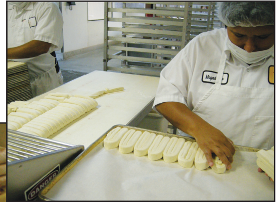
▲ Sheeted, laminated dough is folded, guillotined and then placed on trays to rest before freezing.
