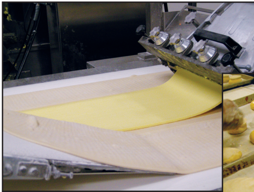
▲ A continuous layer of butter is extruded then folded into the sheeted dough prior to lamination.
