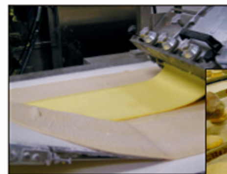
▲ A continuous layer of butter is extruded then folded into the sheeted dough prior to lamination.
